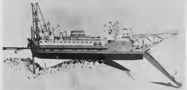
THIS MODEL of the Queen of Holland, cutter suction dredger built last year, illustrates the method of cutting coral which is sucked up to the dredge where it is loaded aboard self-propelled hopper barges.
